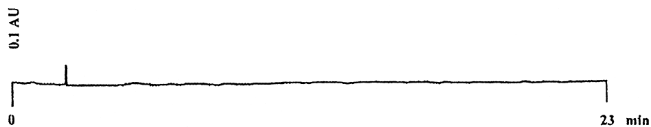
Figure 1. Chromatographic condition on LiChrosorb Si 60 column; mobile phase n-hexane/dichlormethane (10/90 v/v); flow rate 2 mL/min; column temperature 25°C; UV detection at 285 nm, where the peak of dazomet was retained.
